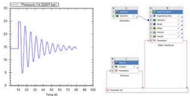
providing the user with the resulting pressure distribution all along the 2-km discretized pipe, at every time-step simulated.
