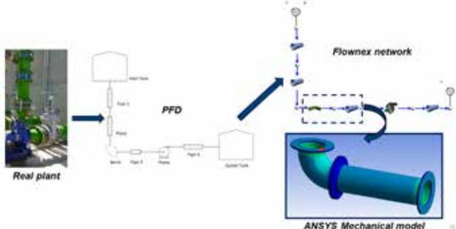
tripping or valve closure. Generally speaking, Flownex is a Computational Fluid Dynamics (CFD) system simulation software that solves equations for conservation of mass, energy, linear and angular momentum. Its fundamental approach is based on a thermal-fluid network of 1D flow components, together with two-dimensional rotating components, and heat transfer building blocks. The solution is calculated with an implicit and fast steady-state and dynamic solver.
