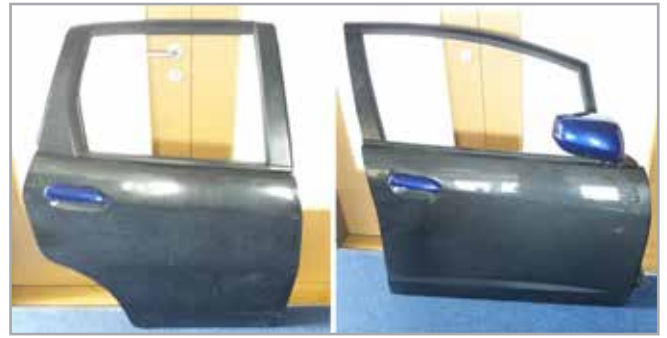
Fig. 3 - A manufactured prototype of the composite side doors of QUIET project
