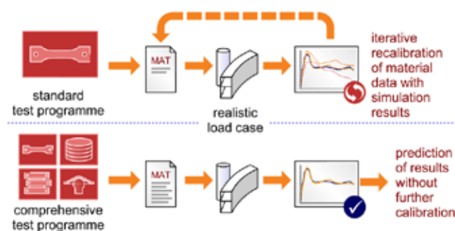
Fig. 1 - CAE development process for crashworthiness based on a simple material model (top) and based on a comprehensive material model (bottom)
