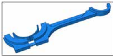
Fig. 6 - 3D solid quarter model and 2D plane stress and strain models.
